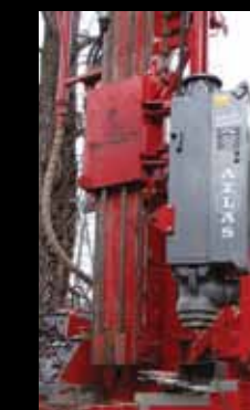
Power Swing out moves hammer away from drill area.
