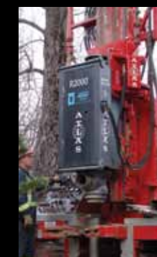
Power Swing out moves hammer away from drill area.
