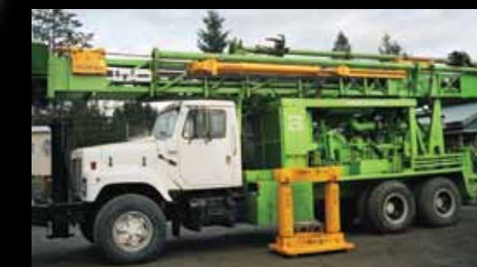
Complete with Atlas Hammer, Lifting Cylinder, Swing Jib and 250 Ton Casing Jack installed at the Atlas Factory.
