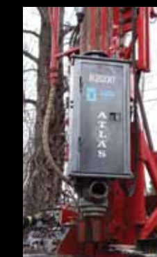
Power Swing out moves hammer away from drill area.
