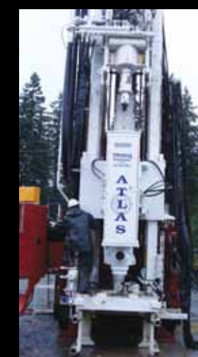
Atlas Casing Hammer on a Power Swing Out system mounted on Schramm T90XD Rig.
